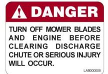
Located on blower, Always turn off mower blades and engine befor clearing discharge chute of serious injury will occur. Discharge Chute be in place when the blower is removed from the mower.
